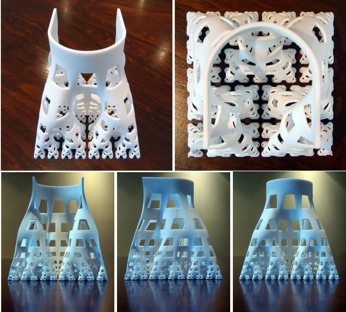
Figure 16: The developing Hilbert curve up to level 4 (constructed by direct parameterisation) as a 3D print.
