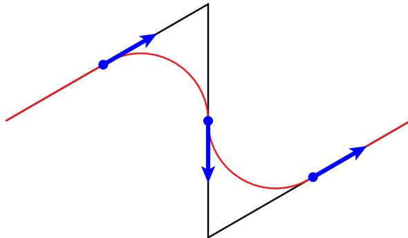
Figure 7: Smoothing a polygonal curve using cubic Bézier curves.
