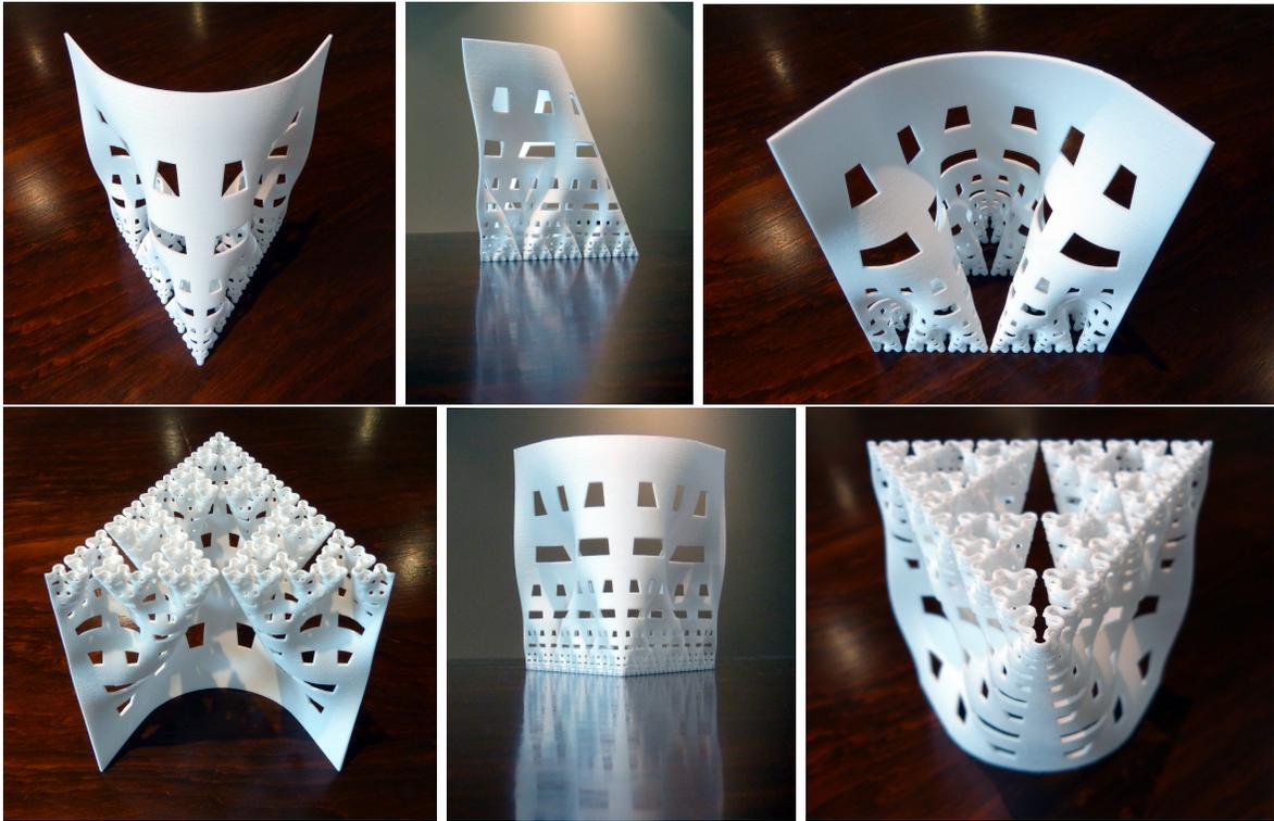
Figure 17: The developing Sierpinski arrowhead curve up to level 6 (constructed by direct parameterisation) as a 3D print.
